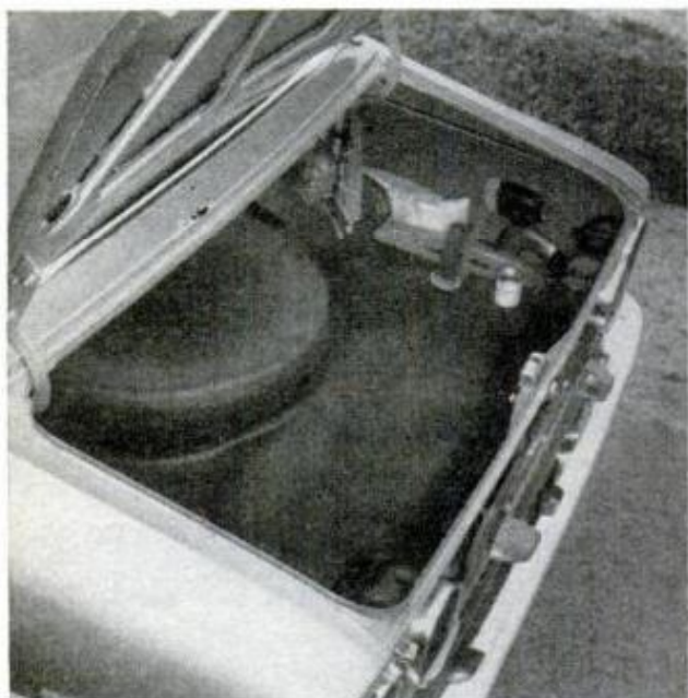
GAS TANK is mounted high behind rear seat, spare tire in its own well, so trunk is square, uncluttered
